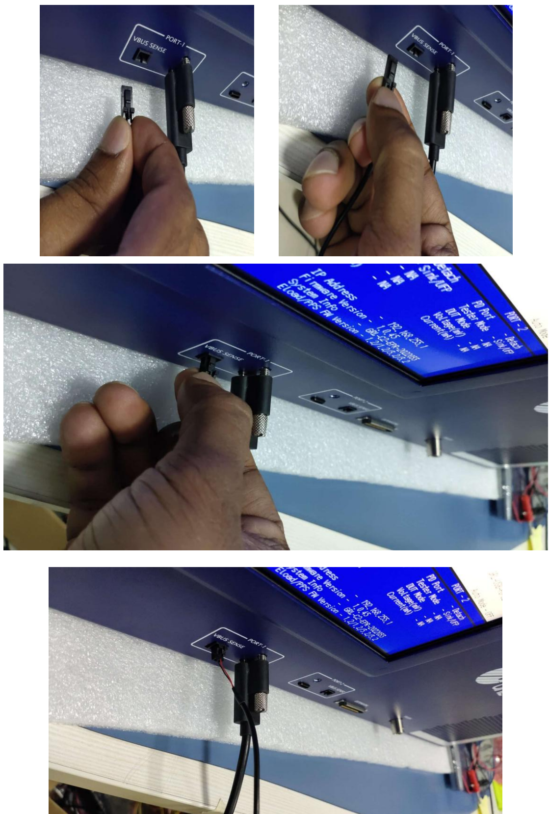
FIGURE 5.12: CONNECTING VBUS SENSE PIN TO GRL-C2-EPR PORT
