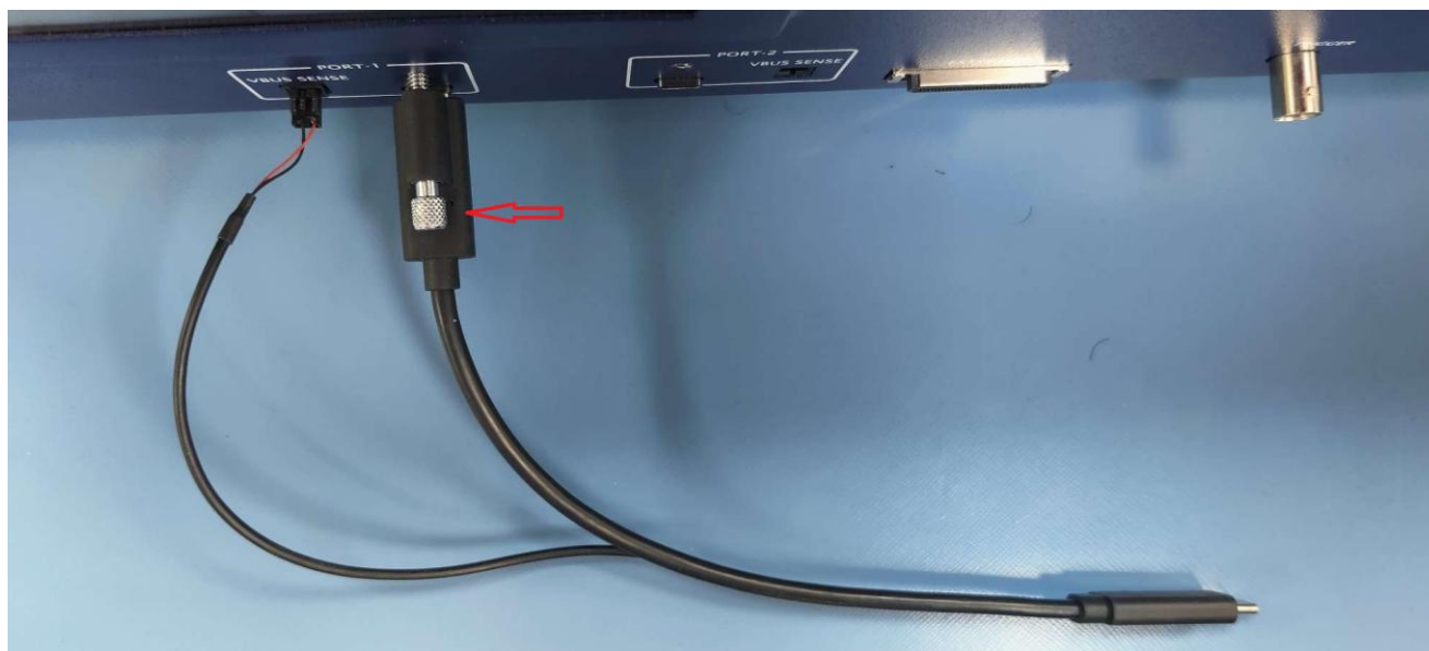
FIGURE 5.9: GRL-SPL-EPR CABLE CONNECTION
