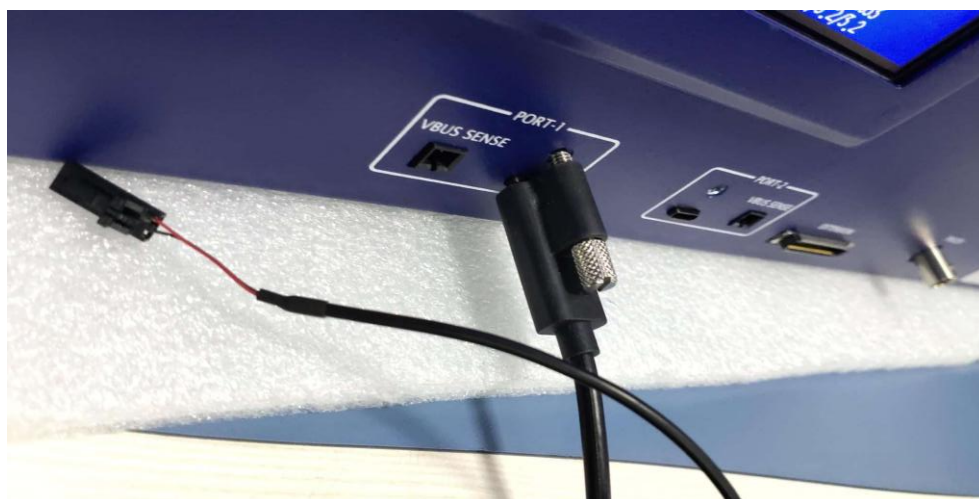
FIGURE 5.11: CONNECTING USB TYPE-C CONNECTOR OF GRL-SPL-EPR CABLE TO GRL-C2-EPR PORT
