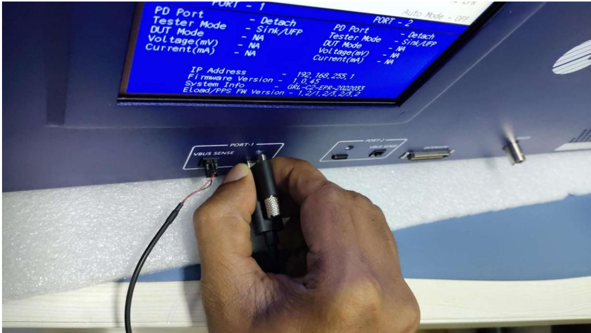
FIGURE 5.13: REMOVING USB TYPE-C CONNECTOR OF GRL-SPL-EPR CABLE FROM GRL-C2-EPR PORT
