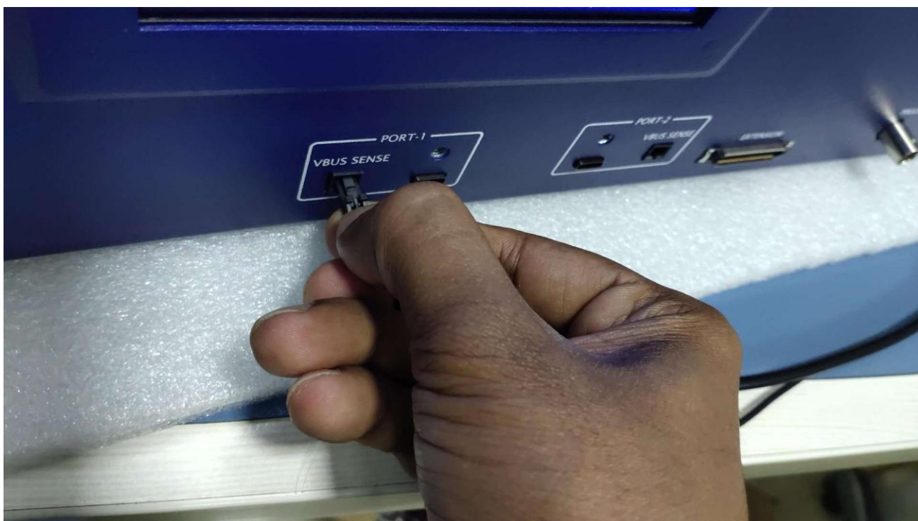
FIGURE 5.14: REMOVING VBUS SENSE PIN FROM GRL-C2-EPR PORT
