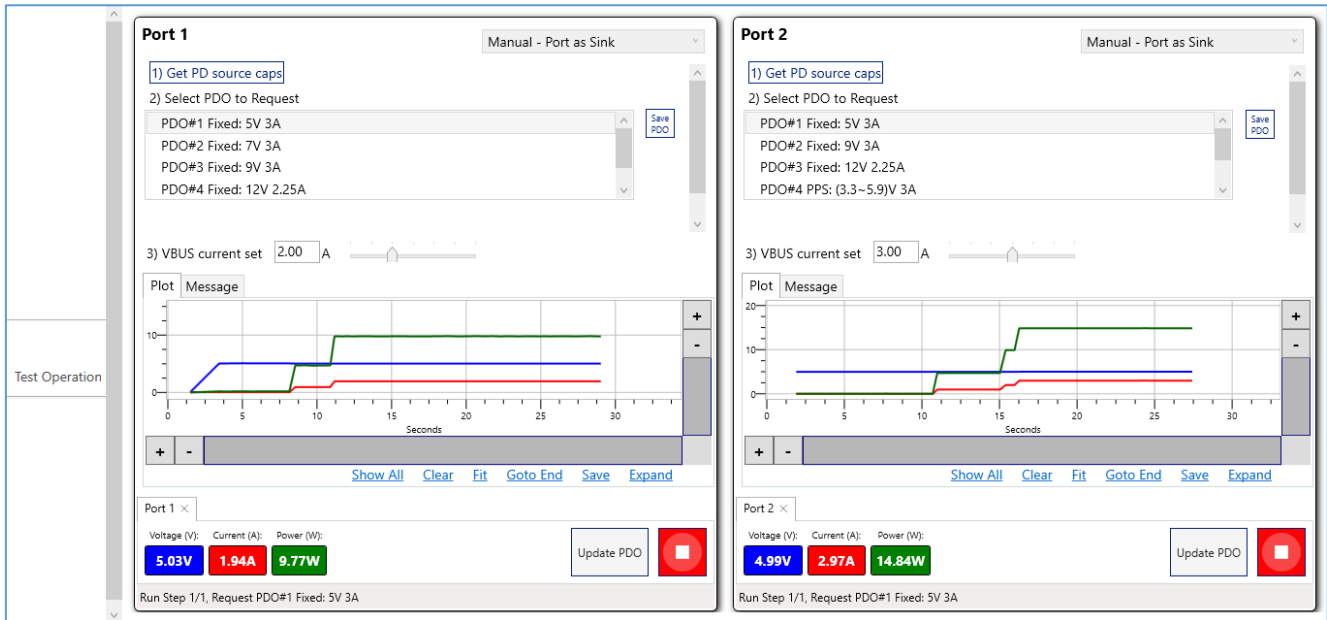
FIGURE 5.4: PERFORM MANUAL CONTROL – PORT AS SINK TEST FOR PD SOURCE UUT
