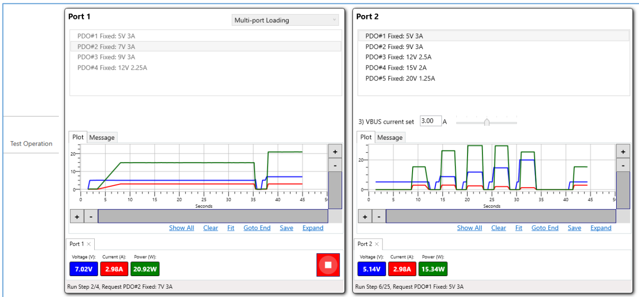
FIGURE 5.25: VERIFY POWER LOAD PER SOURCE PORT OF MULTI-PORT UUT
