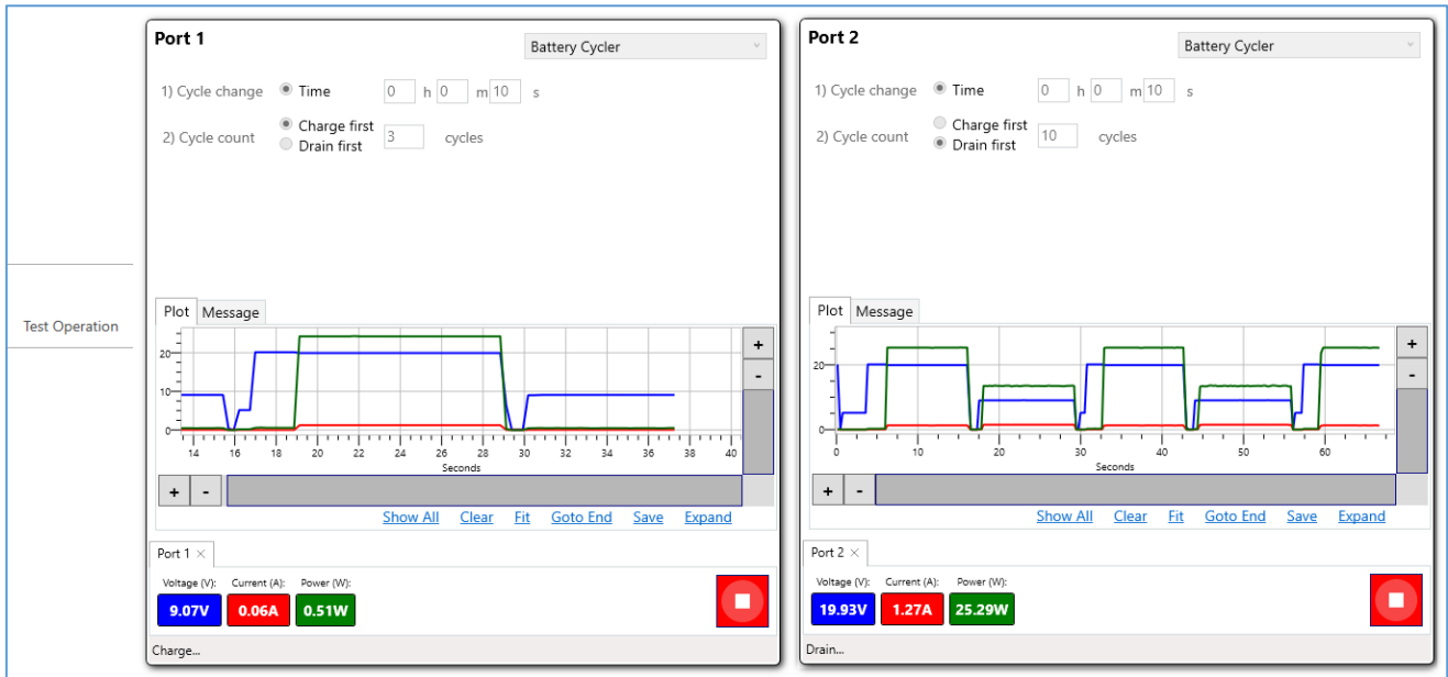
FIGURE 5.22: PERFORM BATTERY CYCLING FOR DRP UUT
